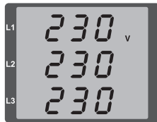
Fig. Example display: Mains voltage per phase
