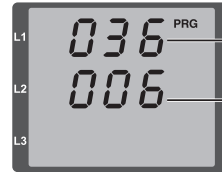
Fig. Example display in "Parameter" programming mode (for Modbus addresses up to approx. 800)
