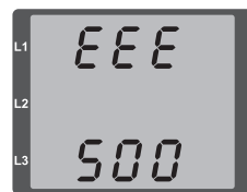
Fig. Error 500 (mains frequency)
