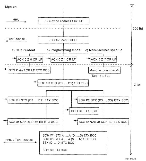
Figure 12 - Diagram protocol mode C
