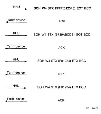
Figure 22 - Example of a partial block formatted write
