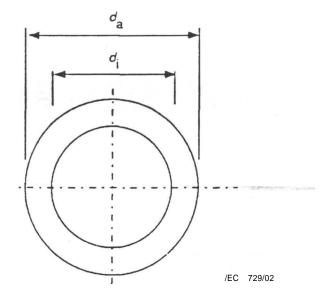
Internal diameter  $d_i$  - 13 mm ± 1 mm: External diameter  $d_a$  - 28 mm minimum Magnetization: axial, north pole directed towards the tariff device.
