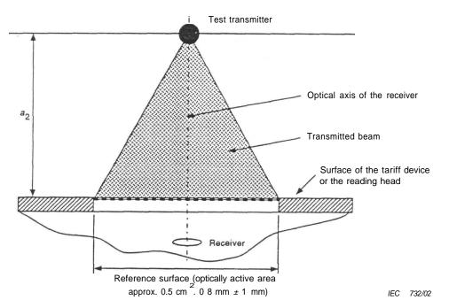
Figure 6 - Test arrangement for the receiver
