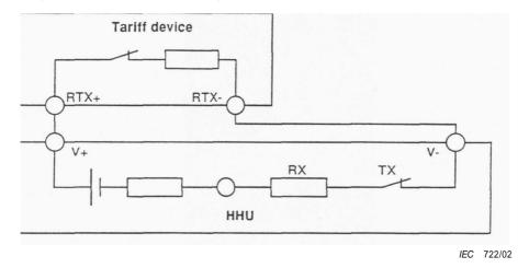
Figure 1a - Circuit diagram of a two-wire single slave configuration
