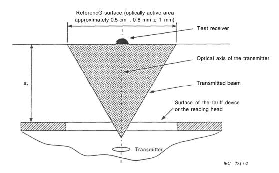
Figure 5 - Test arrangement for the transmitter
