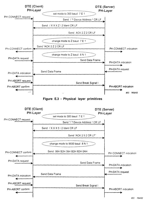
Figure E.4 - Physical layer primitives, simplified example with one mode change only
