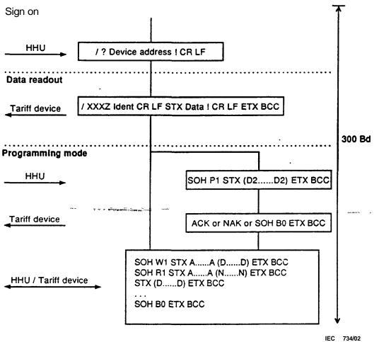
Figure 8 - Diagram protocol mode A
