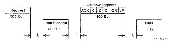
Figure 14 - Transmission protocol for protocol mode C giving data readout with confirmation of the suggested baud rate
