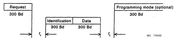
Figure 9 - Transmission protocol for protocol mode A
