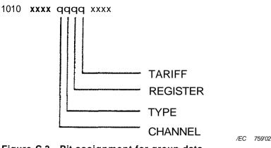
Figure C.3 - Bit assignment for group data
