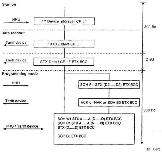
Figure 10 - Diagram protocol mode B
