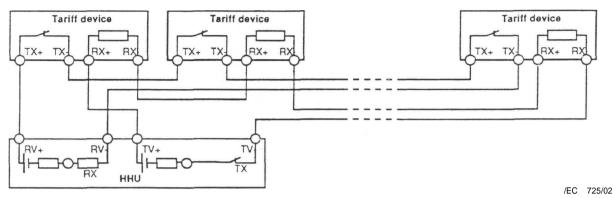
Figure 1d - Circuit diagram of a four-wire multiple slave configuration
