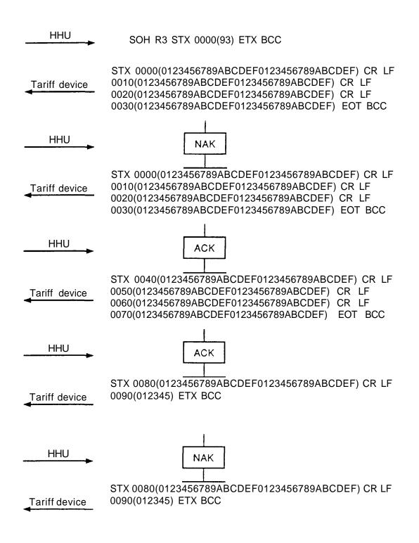
Figure 21 - Example of a partial block unformatted read
